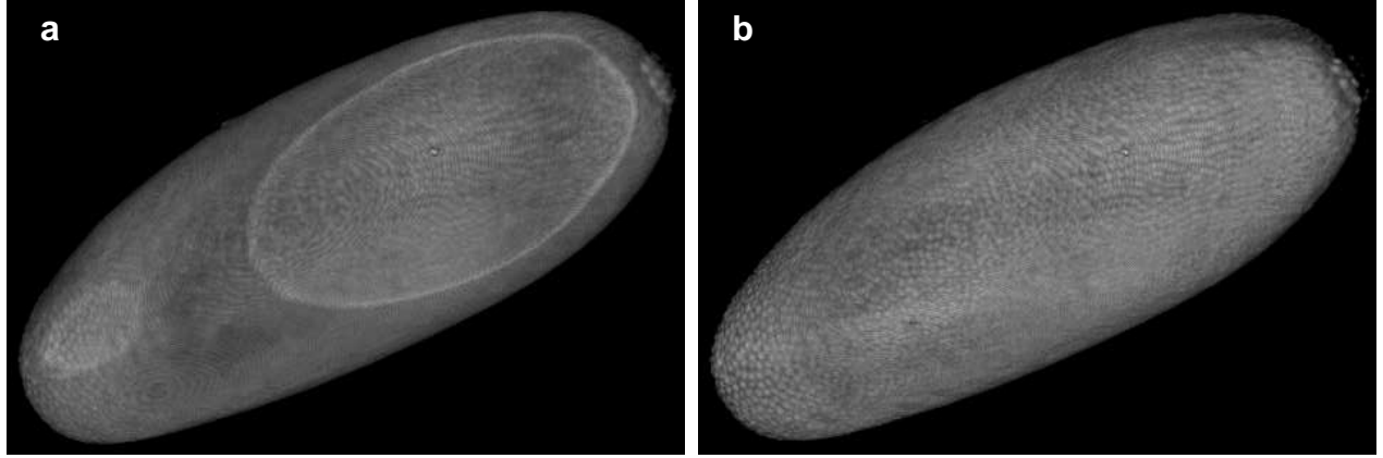
Figure 7. Illustration of truncation artifact that is removed by content-based image fusion. (a) Due to the truncated acquisition of one of the eight views, volume rendering the result of simple averaging shows a clear artifact in the shape of an ellipse. (b) The artifact is removed by the content-based image fusion, due to the low information content of the image region in the truncated view near the truncation surface.
